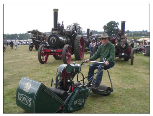
My name is Dennis and I have a 24 inch cutting cylinder and a matching sit-upon roller seat that my current owner sits on to steer me and show me off! My impressive single cylinder 4-stroke side valve engine has a capacity of about 640cc and will keep me cutting grass all day without sweat.
