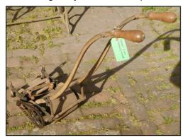
tations of width, pitch and roller diameter. This one needed to be half an inch wide, and half an inch in pitch. The width is measured between the inner link-plates, and the pitch is the centre-to-centre distance between the pins. Alas,  $\frac{1}{2}$  x  $\frac{1}{2}$  in. is not among the many currently available sizes. So the Caledonia, a 12-inch with grassbox, remained chainless.
