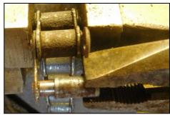
above left). If I had been really keen, I could have made a special semi-circular punch to fit against the perimeter of the roller (which is what I am calling the outer sleeve), but I managed with an ordinary round pin punch, applied at intervals round the joint, although its localised force tended to distort the plates, and I found that a screwdriver was better. It had a plastic handle, and survived the ordeal unscathed.
